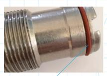
Particular attention needs to be paid to sealing areas ensuring that no damage is present that can compromise the integrity of the O-Rings. Delavan strongly recommends the replacement of these O-rings each time the nozzle is assembled.
